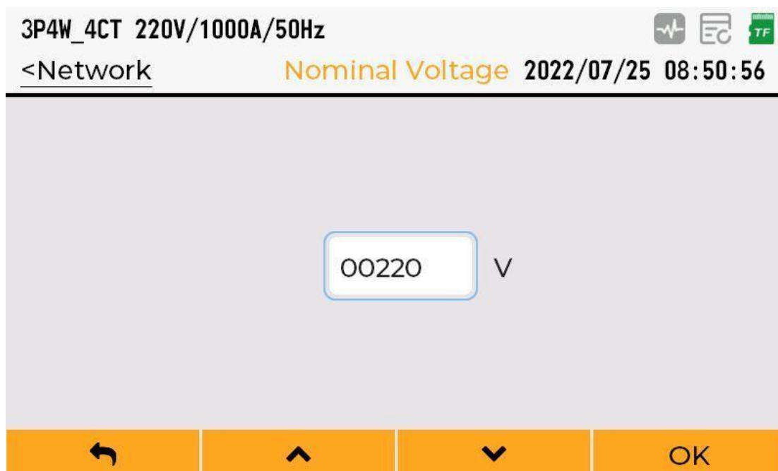
Figure 5-7 Nominal voltage configuration
